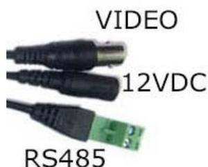
**BNC video output** - At the BNC bayonet socket connecting the video cable which then leads to a AHD DVR.
